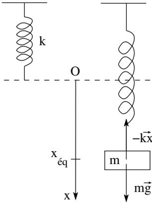
Figure 5.5 – Masse oscillante suspendue
